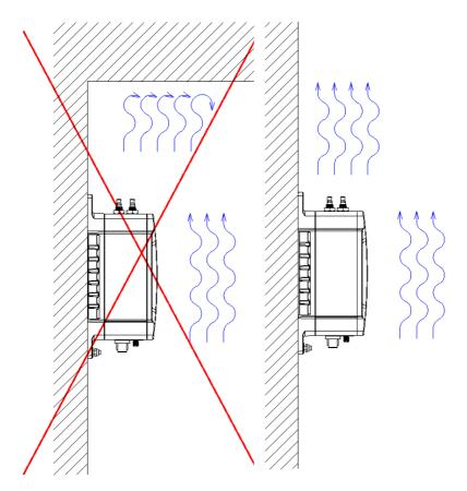
Figure 8. Installation with reduced natural convection airflow
