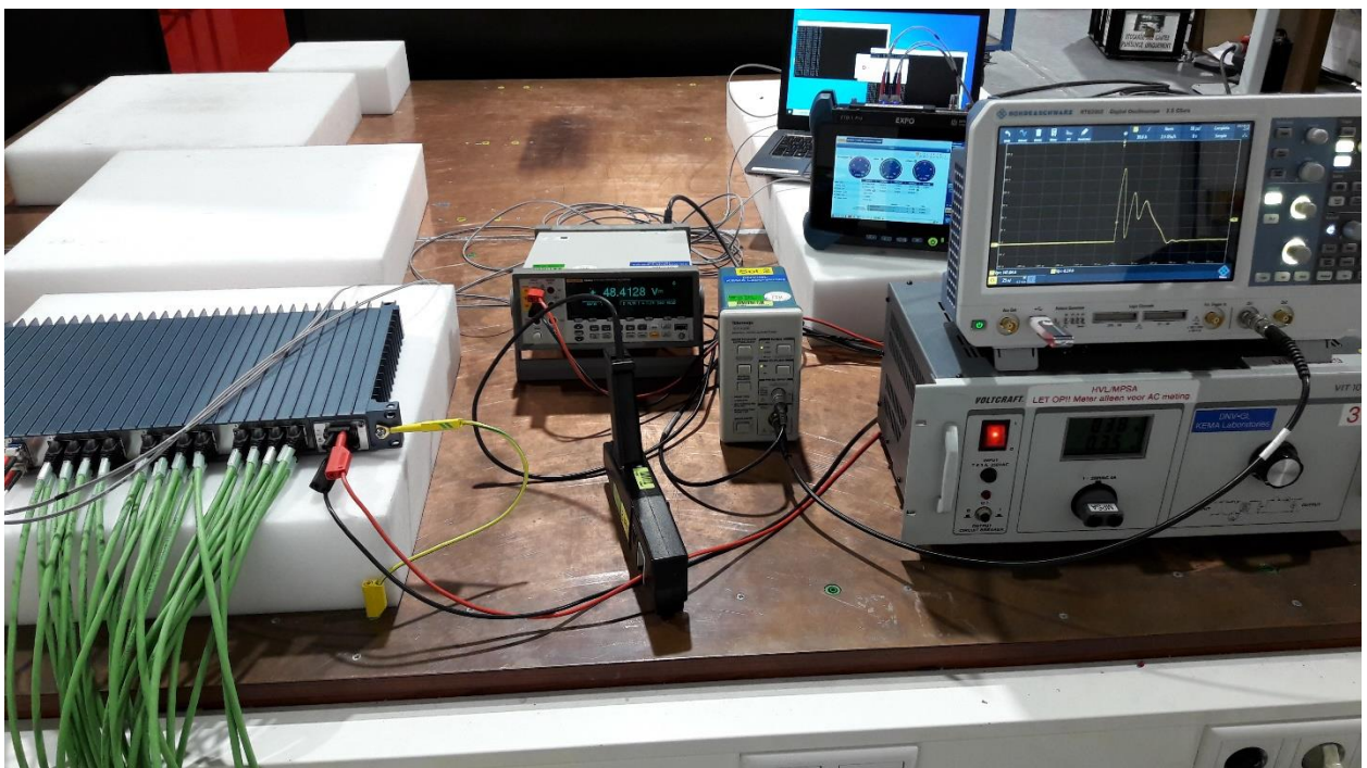
Photo test arrangement inrush
