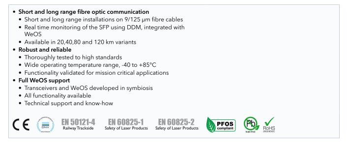
Westermo's 100 Mbit/s singlemode SFPs are suitable for short- and long-range applications. The available models can use singlemode fibre cables with a core of 9  $\mu$ m. Using the DDM functionality, which is fully integrated into WeOS, it is possible to monitor parameters such as temperature, TX/RX power, and voltage, ensuring correct operation.
