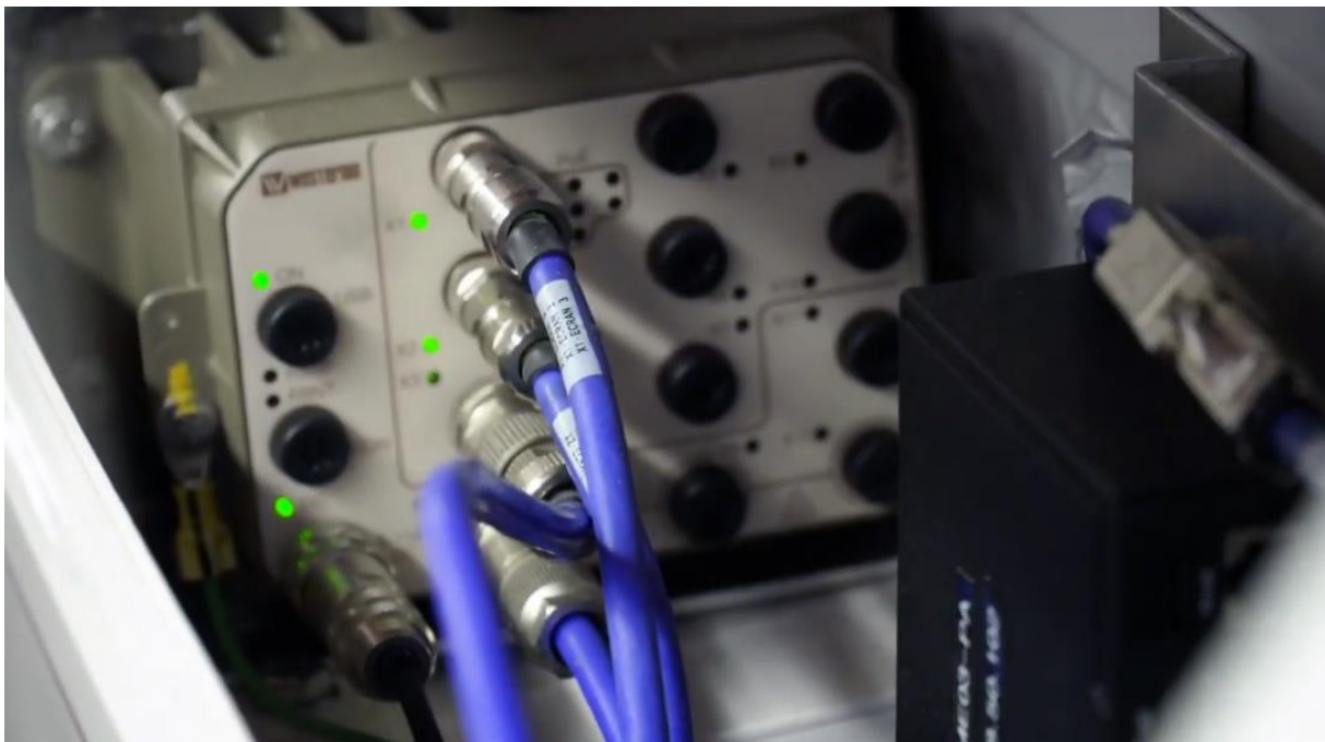
The Viper switch in the confined space onboard the ORLYVAL shuttle. Picture credit: RATP Group
